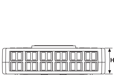
Front View of 24 core LC Cassette with MTP connectors on rear
