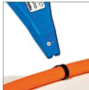
Bring the tool perpendicular to the tie...
